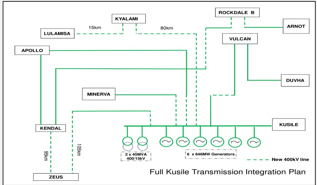
**Figure 6.6.2: Kusile Power Station Integration single-line diagram**
