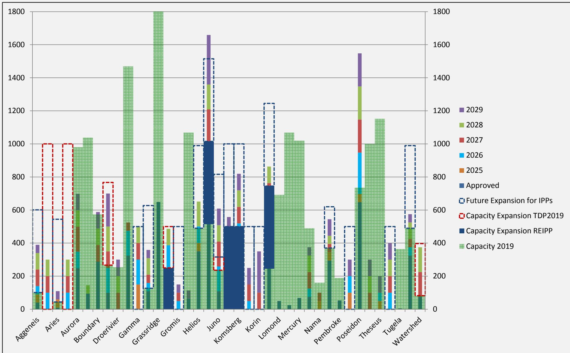
Figure 7.5: Transformer capacity enhancement for IPP integration- TDP 2020 - 2029
