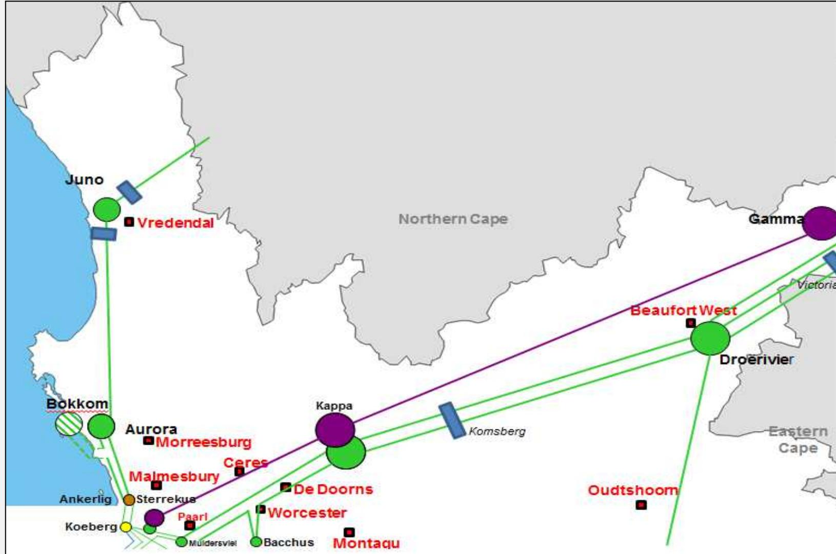
Figure 6.9.1: Current Western Cape network diagram
